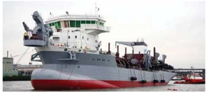
Self-propelled seagoing hopper dredge.
