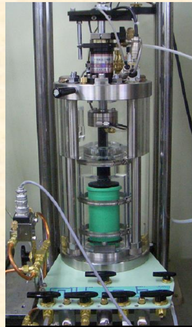
Triaxial compression device for unsaturated/saturated sample with double-cell type volume meter (Axial translation method)
