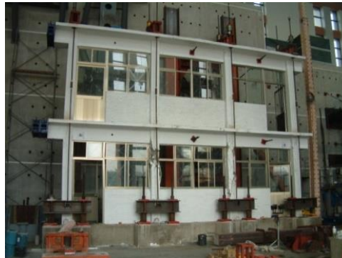
A full-scale test of school frame in lab
